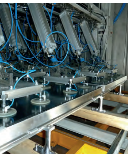
Shear load test of a complete system consisting of two collectors with a mounting system, including connection to the load-bearing structure up to the roof rafters.
