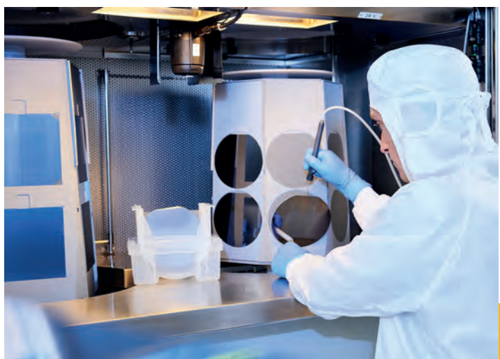
Wafer handling for the Si epitaxy reactor.
