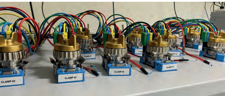
Personnel air lock for changing into and out of personal protective clothing (above); Processing of powders, mixing of electrode slurries and products of novel, silicon-based active materials (center); Cycling of lithium-ion test cells in a cell tester (below).
