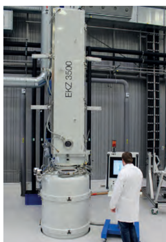
Czochralski facilities for producing monocrystalline silicon ingots (left) and silicon monocrystals (right).
